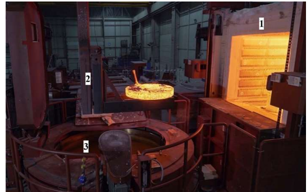
Figure 3. Transportation of the hollow disk.
