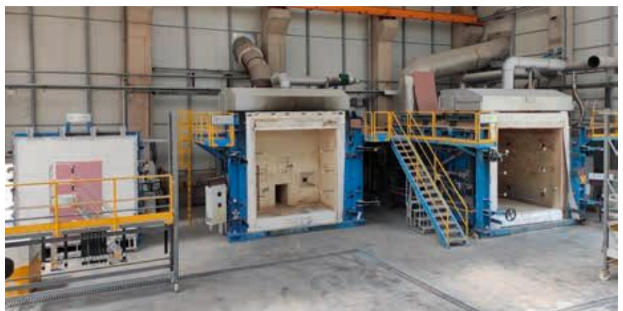
▲ Efectis's knowledge about fire testing over 70 years and the knowledge of industrial furnaces of Sistem Teknik were combined and Turkey's first fire resistance test furnace was produced.
