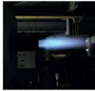
Ratio of natural gas/hydrogen 20/80
