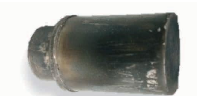
▲ No wear and sticking issue was encountered after 40K presses with BÖHLER W360 ISOBLOCK. (W360 ISOBLOCK)
