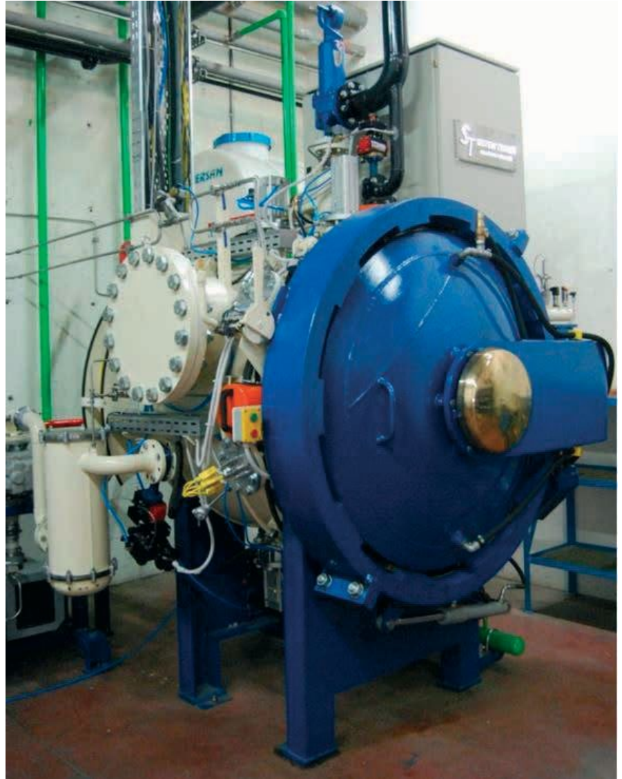
▲ Figure 1 Vacuum Carburizing and High Pressure Gas Quenching
