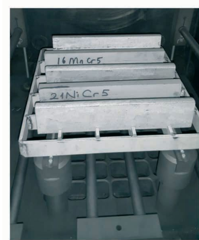
Figure 3 Samples after the carburization
