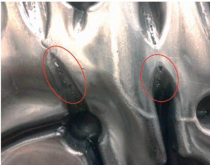
▲ 1.2343 ESR steel that we had to maintain due to thermal cracks and breaking after 20K presses
