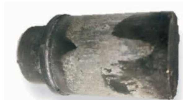
▲ Sticking and wear issues were experienced in the area opposite feeder input (1.2343 ESR and different surface coatings)
