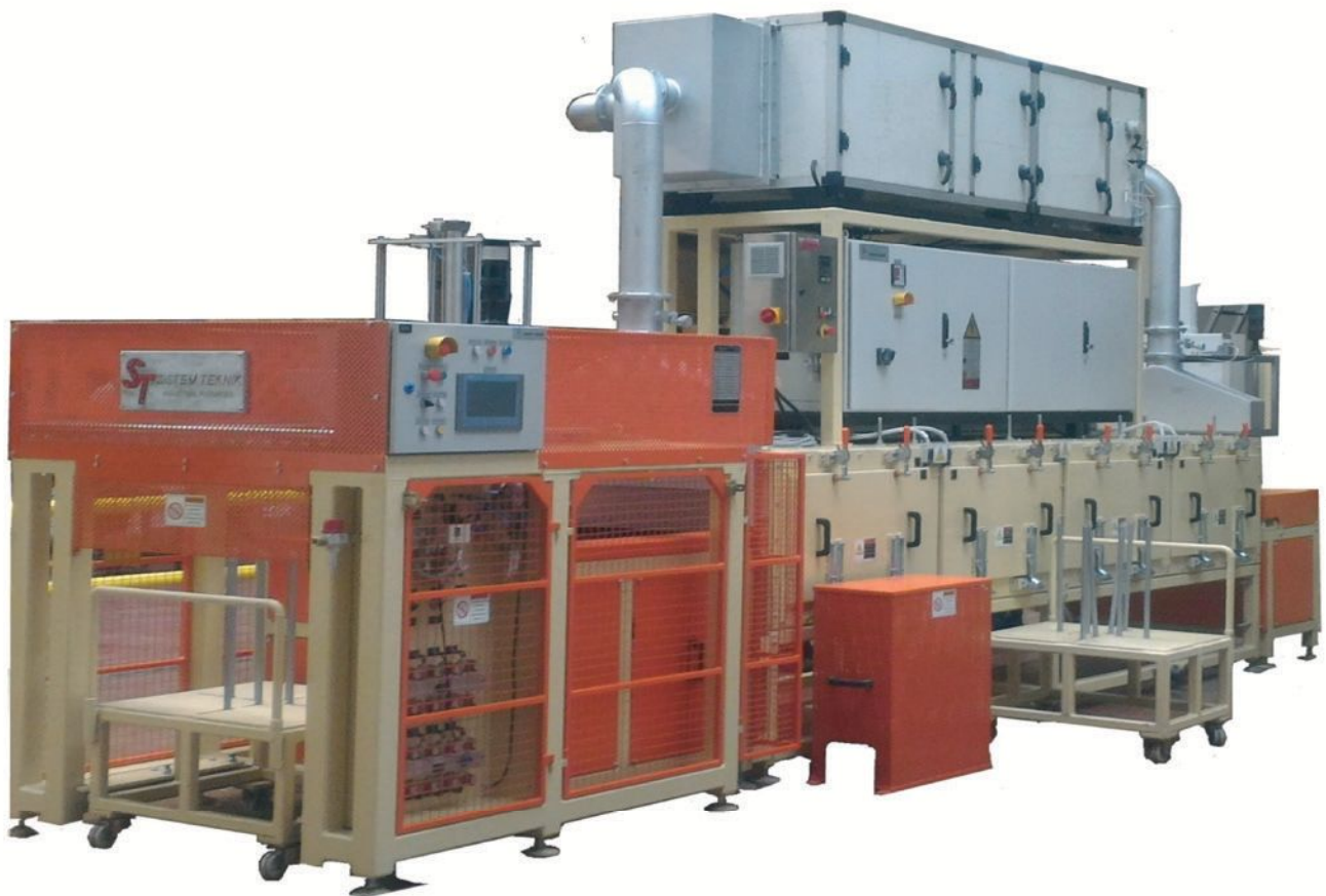
▲ Figure 4- Infrared Furnace.
