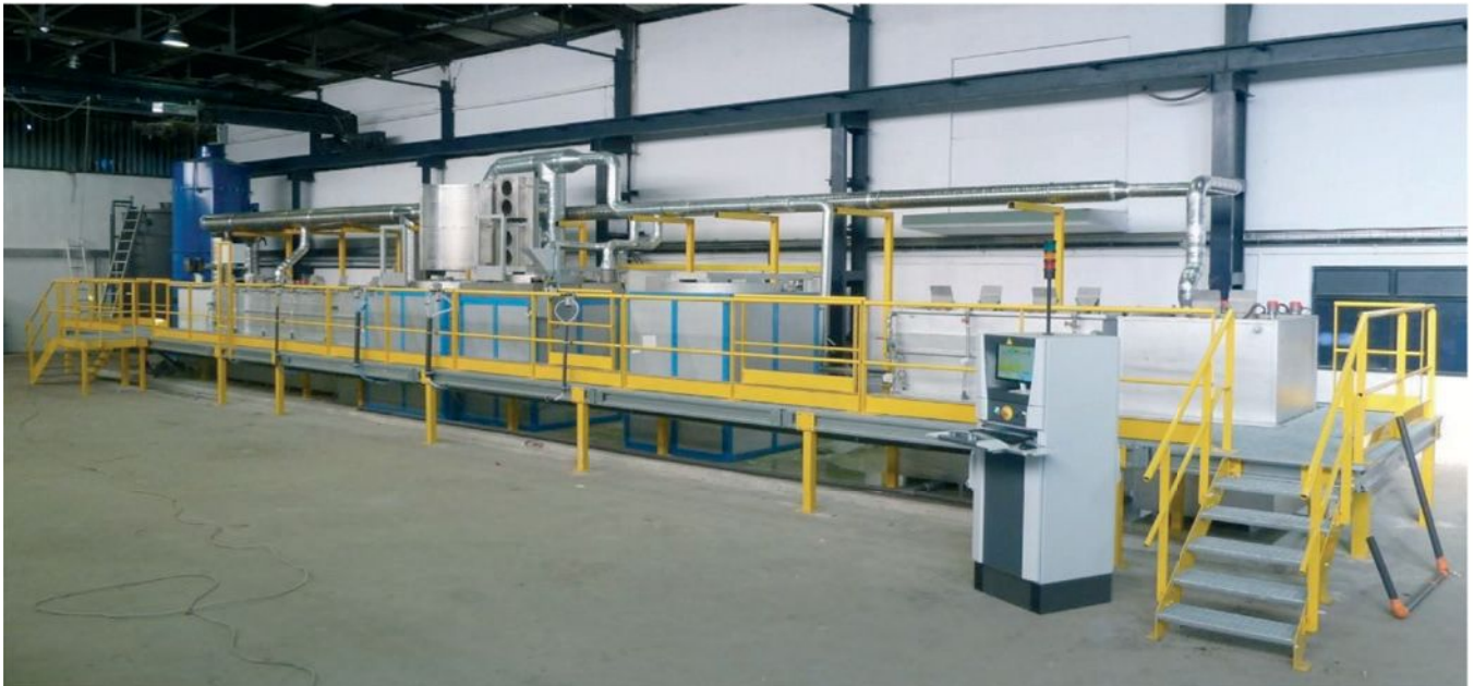
▲ Computer-controlled salt bath plant for carrying out the TUFFTRIDE QPQ process
