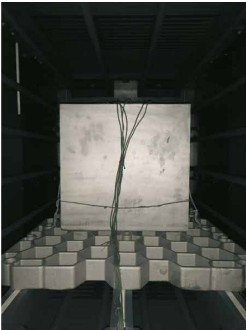
▲ Figure 5. Test Block After NADCA Test
