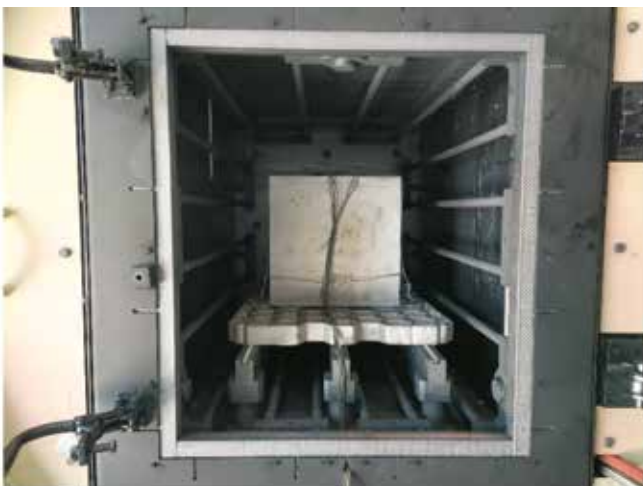
▲ Figure 1. Placement of NADCA Test Sample in the Furnace
